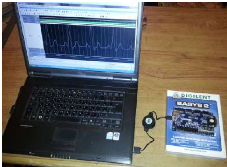
Figure 2: The design is implemented on FPGA board (XC3S250E) with a usb interface to provide the flexibility to adjust the ECG signal.
